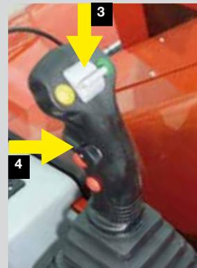
3. Tillaging roller rotation speed adjustment to variable r.p.m. according to the type of product to be tillaged.
