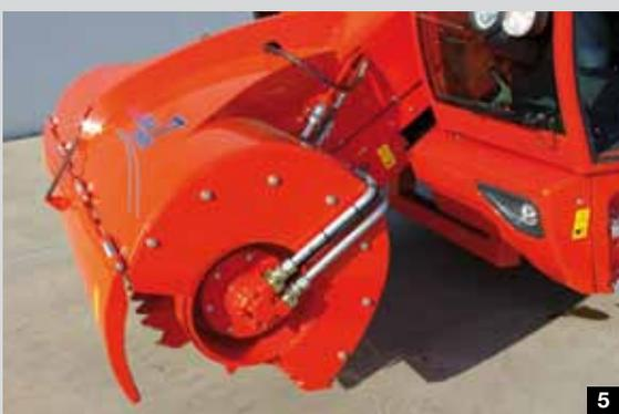
5. Tillaging roller diameter 400 mm, driven by 2 hydraulic motors, power 110 kW, rotation speed 0:670 rpm.
