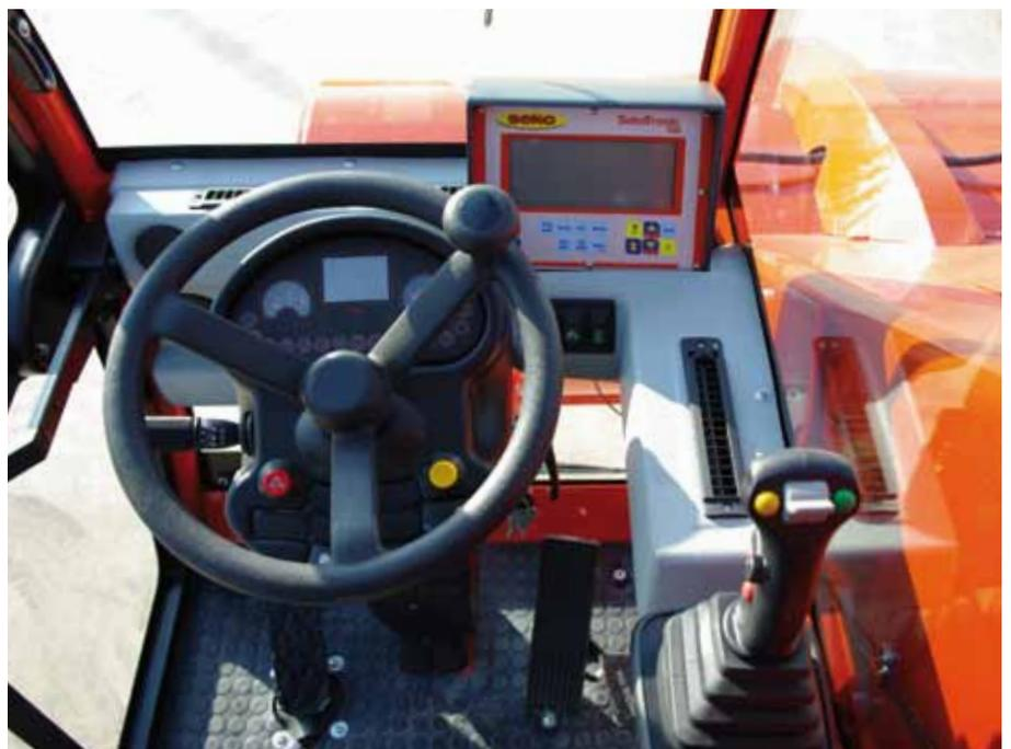
Dependable and advanced weighing and data transfer systems allow programming of different recipes according to the different types of livestock, and constant monitoring of the ration in the display and in the farm management system.
