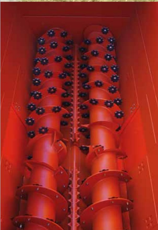
Our patented “Double Mix” chopping and mixing system is characterised by two special double spiral counter-rotating augers housed on the bottom of the box, provided with star-shaped knives and counter-blades for processing any product, offering limited power absorption and high performance.
