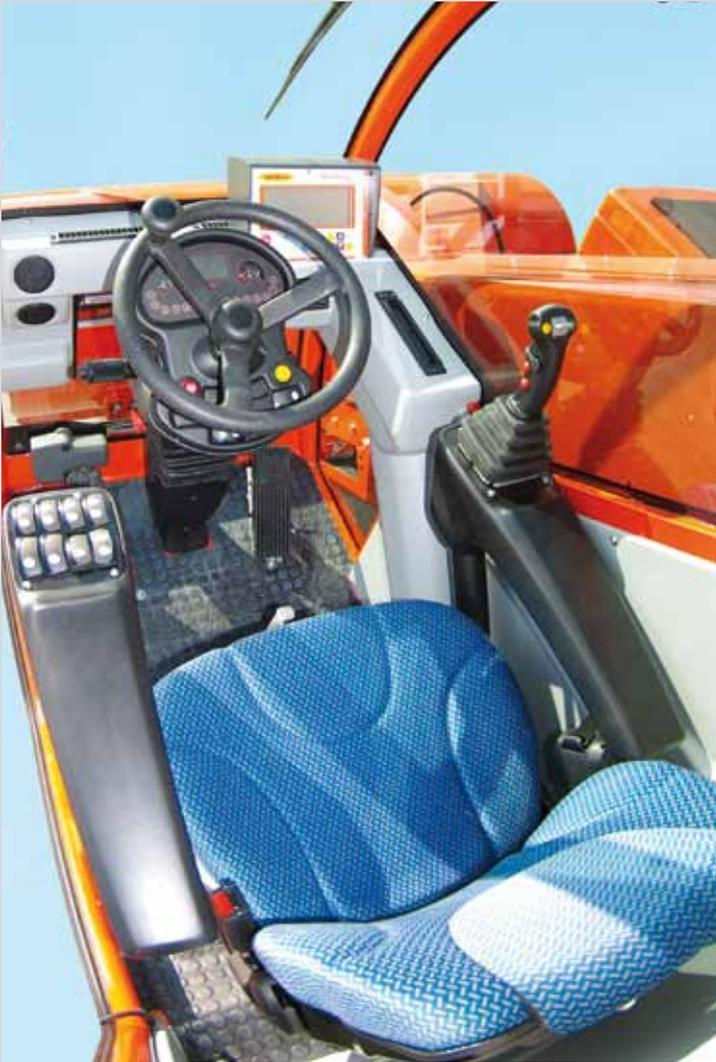
For greater driving comfort, all the main controls (travelling transmission + silage tiller operation) have been incorporated in a practical joystick integrated in the right-hand arm of the seat, while all the manual controls of the machine are operated from the left-hand arm.
